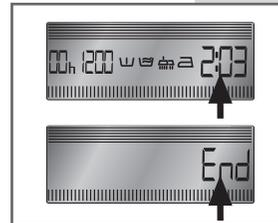
**DELAYED START:** This function allows the start of the wash cycle to be delayed by up to 16 hours. Press button **B** repeatedly until the required delay time appears on the display. Icon h will flash on the display until the wash cycle starts.
