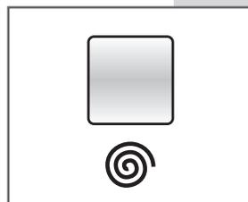
**PRE-WASH:** To carry out a prewash, press button **D** and add detergent to the appropriate compartment **1**. The washing machine will carry out a prewash at 40°C max. A Prewash is recommended for items soiled with dust, soil, sand or with particularly resistant stains. See the Programme Table for further information.
